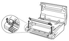
4. Release the guide by pulling it in the direction of the arrow.
